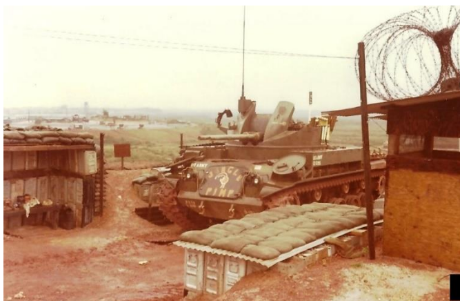
Duster in fortified firing position showing twin guns and unpacked, clipped ammunition stacked around the “tub” up top. Sand-filled ammo can protection is visible, with concertina wire on top of hooch to dissuade sappers and disperse any incoming mortars.
