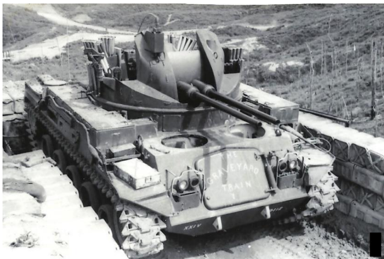
Duster in a fortified firing position at Firebase Birmingham showing twin guns and unpacked ammunition stacked around the circular gunner and crew “tub” up top.
